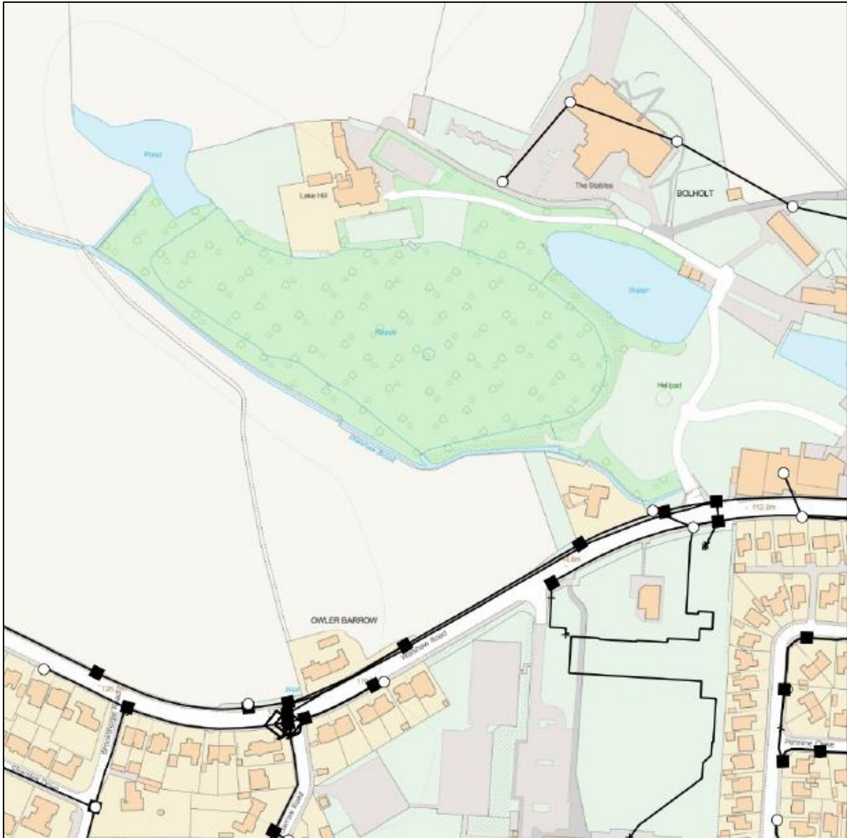
Figure 10 – BT Openreach Infrastructure Records Central
